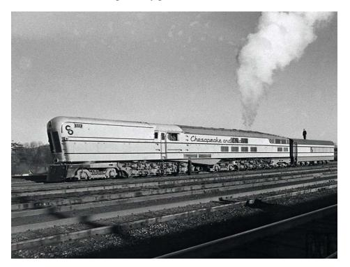
No. 500 with a full head of steam. The coal bunker is in the front of the locomotive and the 25,000 gallon water supply is trailing in a specially built water tender designed to match the passenger cars. The fire box is located behind the crew's compartment. Built in 1947-8 the three locomotives proved unsuccessful and were sold for scrap in 1950.
